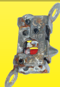
Zinc plated steel fire detection mechanism after 240h salt spray at 20%
