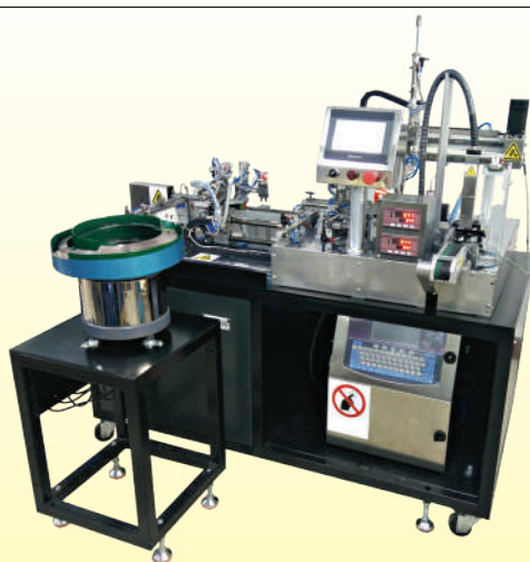
Automated testing of the solder strength in production at ambient temperature
