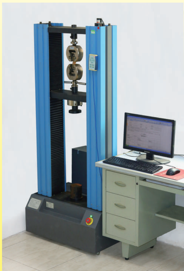
Tensile strength and elongation at break equipment
